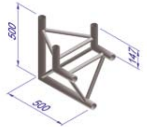
type description 006 2 way corner 90° apex up
